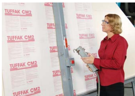
Figure 1. Author Liz Grimes uses a vertical panel circular saw to cut a large polycarbonate sheet. The panel saw is the best choice for sheet thicknesses less than 0.118 inches.
