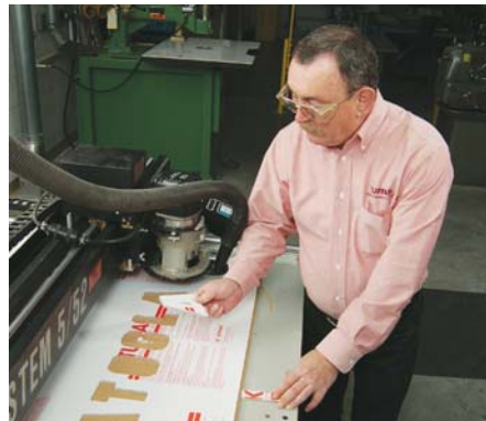
Figure 5. Atoglas Technical Assistant James Eastwood operates a computer controlled router, which follows an electronic template to create complex shapes in polycarbonate sheet.
