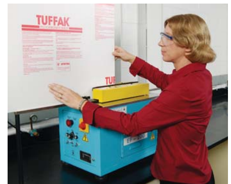
Figure 6. Liz Grimes achieves a smooth, glossy edge in Tuffak® polycarbonate sheet with an automatic edge-finishing machine outfitted with a diamond-tipped spindle.
