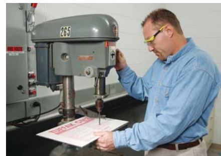
Figure 3. A modified 118° point angle twist drill bit for polycarbonate sheet provides optimum drilling. Atoglas Technical Assistant Gary Hall drills a slightly oversized hole for a fastener in this polycarbonate sheet.
